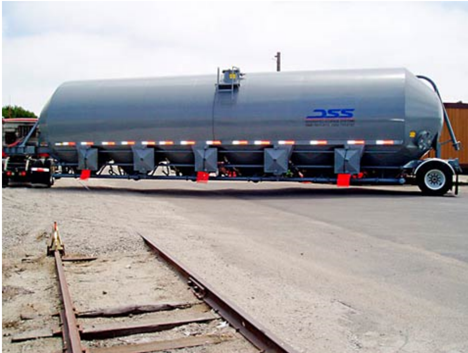
Figure 11: 4200 cf (~150 cy) capacity cement guppy.
