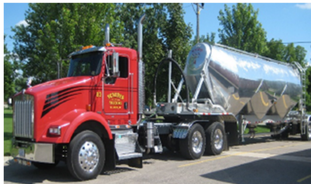
Figure 1: Dry bulk tanker truck. This is the type of truck that will haul the cement and fly ash up to the site.
